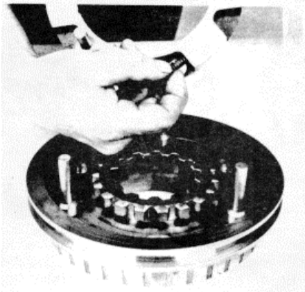
(2) Install the three springs in the bores of the direct ring.
