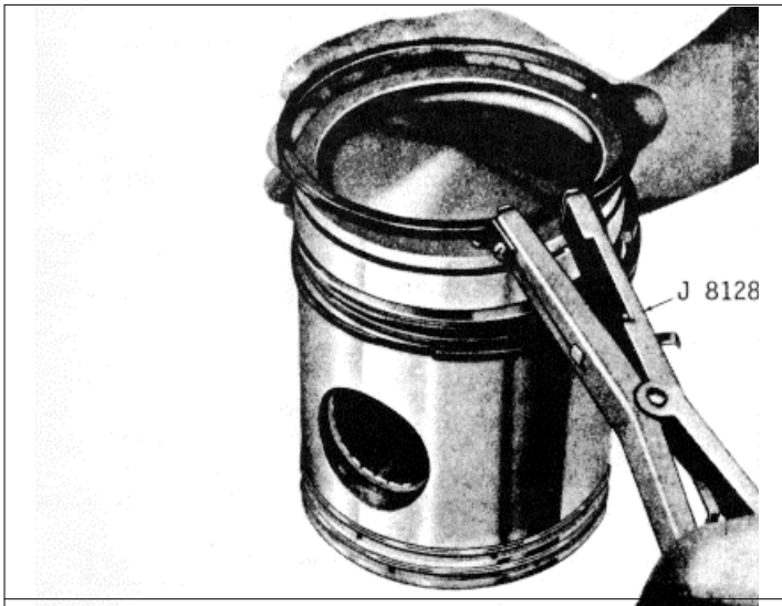
Fig. 3 Removing or Installing Piston Rings 19.4 Cleaning
