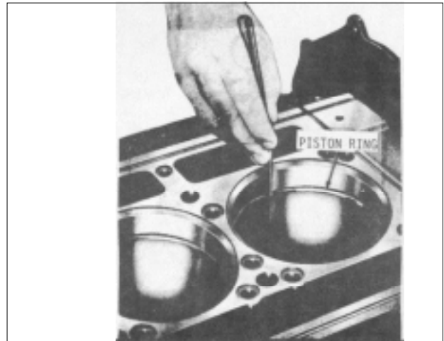
Fig. 14 Measuring Piston Ring Gap
